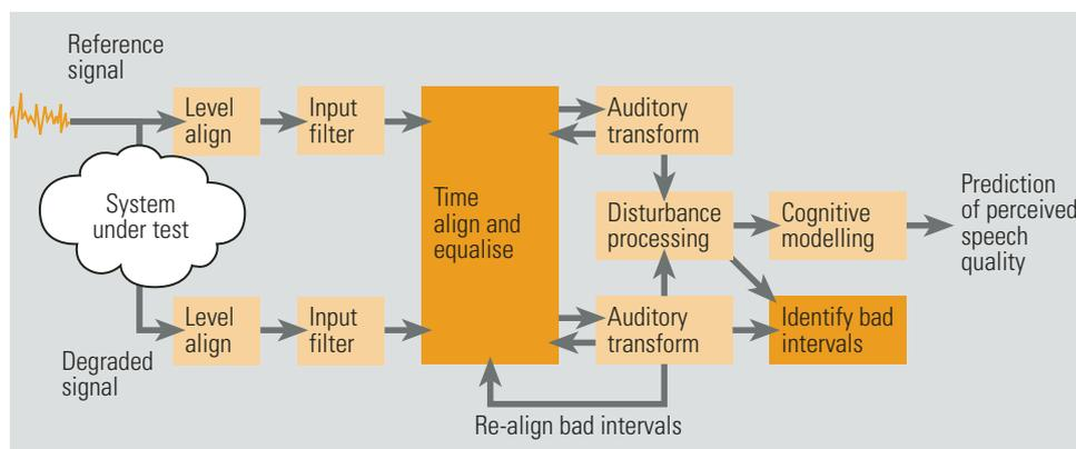
One of the major advantages of PESQ over other measurement approaches is that it does not need to make any assumptions on the network under test or the distortion types that may occur in a specific telephony test scenario. The only prerequisite employed within the model is the scientific knowledge on how human speech is produced and how humans perceive it.
