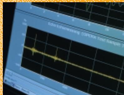
*Our new generation of quality testers, called OPERA™ – short for „Objective Perceptual Analyzer“ – represent the latest development to objectively evaluate and assure the quality of compressed speech and wide-band audio signals by modeling the human ear.*
